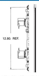
INSTALLATION NOTE: MANIFOLD MUST BE MOUNTED A <u>MINIMUM</u> OF 2-3/4 INCHES FROM FACE OF WALL TO ALLOW FOR CLEARANCE OF SOLENOIDS.
