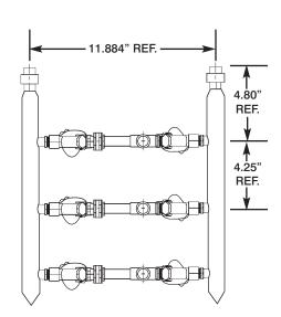
INSTALLATION NOTE: MANIFOLD MUST BE MOUNTED A MINIMUM OF 2-3/4 INCHES FROM FACE OF WALL TO ALLOW FOR CLEARANCE OF SOLENOIDS.
